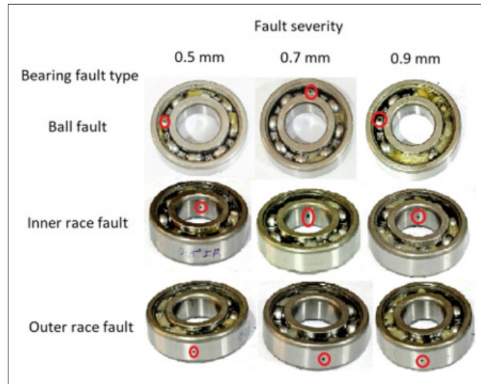
Figure 7: Different types and severities of faults.
